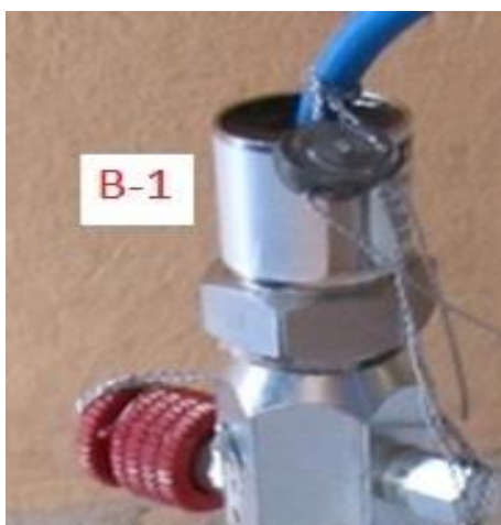
Figure 11: Type B sealing for pressure transducer
