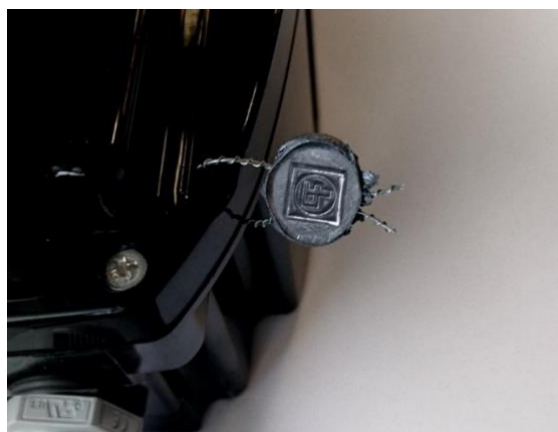
Figure 15: Non-metrological hardware seal on the MODUS lid
