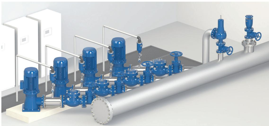
**Reduction units.** Positioned downstream of a reduction unit, the valve protects the main pipeline from uncontrolled pressure increases. The installation includes the H-VAL 310/410 pressure reducing valve, a maintenance bypass and upstream and downstream WAVE or WAVE LITE 3S AWH anti-water hammer vents.
