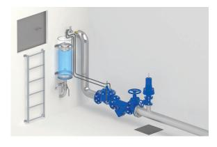
**Level control.** In installations with automatic tank level control valves, particularly when managing minimum and maximum levels, there is a significant risk of overpressure during the closing phase of the valve.
