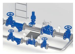
**Quick disconnecting devices.** Positioned upstream of quick disconnecting devices, such as H-VAL hydro valves, the valve prevents pressure build-up following a sudden stop of the fluid column. In these installations, it is recommended to also introduce downstream and upstream triple-acting anti-water hammer vents of the WAVE or WAVE LITE 3S AWH model.
