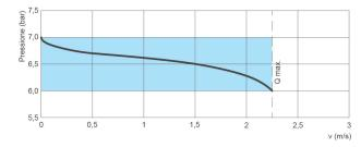
**Valve sensitivity** The curve shown in the figure shows the indicative change in actual downstream pressure from the set value as the flow rate increases. The maximum speed and recommended working conditions are indicated (blue area).
