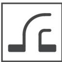
**SUB version**, with conveyance drain, available for WAVE LITE 2S and 3S models. The threaded bend, connected to a discharge pipe, allows the air valve to operate even in the event of flooding of the well or the installation site, without the risk of contaminated water entering the pipeline. Another advantage of the SUB model is the possibility of conveying spurts when the air valve is closing.
